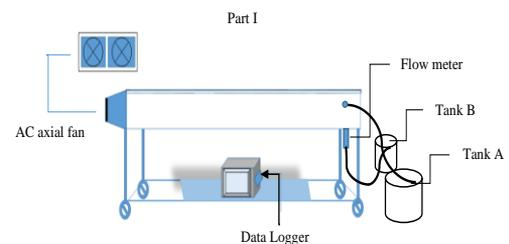
**Figure 2.** Schematic diagram of outdoor experimental setup
