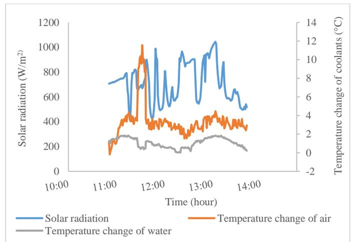
**Figure 4.** Temperatures and solar radiation against time for water mass flow rate of 0.03 kg/s
