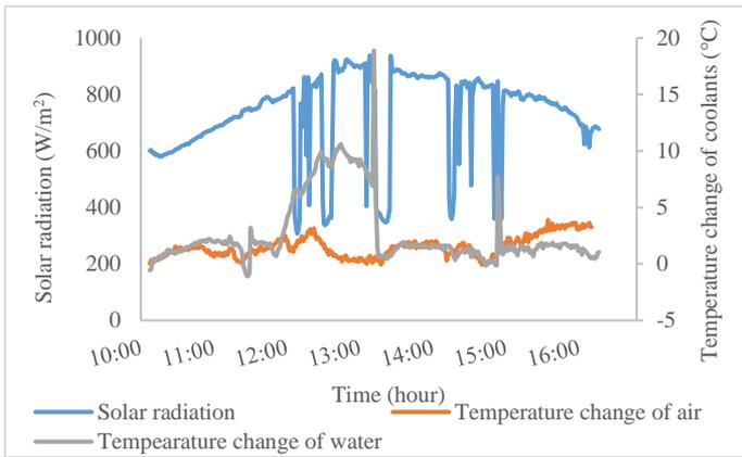
**Figure 5.** Temperatures and solar radiation against time for water mass flow rate of 0.025 kg/s
