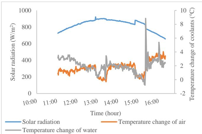
**Figure 6.** Temperatures and solar radiation against time for water mass flow rate of 0.02 kg/s
