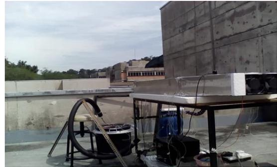
**Figure 1.** The experimental setup of PV with bi-fluid cooling system
