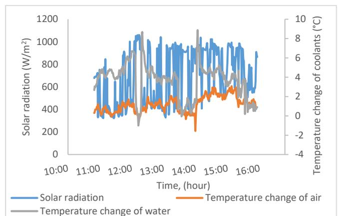
**Figure 8.** Temperatures and solar radiation against time for water mass flow rate of 0.01 kg/s
