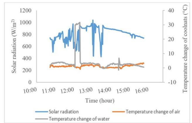
**Figure 7.** Temperatures and solar radiation against time for water mass flow rate of 0.015 kg/s
