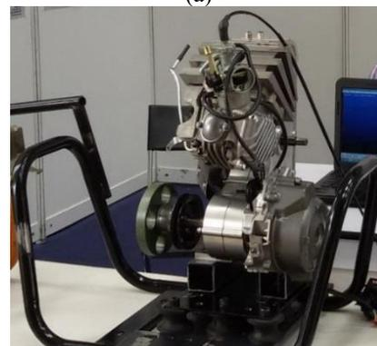
**Figure 1.** (a) Design of Crank-Rocker Engine and (b) Fabricated and Assembled C-R Engine [18]
