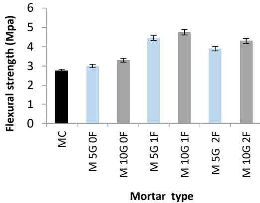
Figure 4. Flexural strength of mortars
