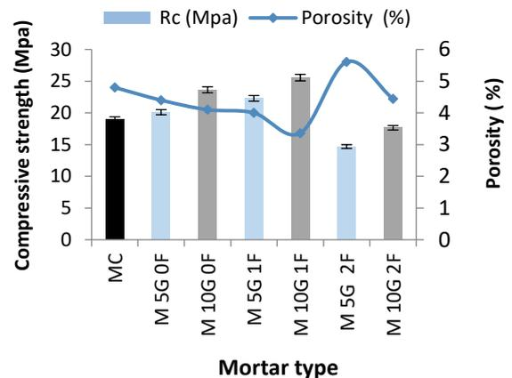
**Figure 3.** Compressive strength and the porosity of the different mortars
