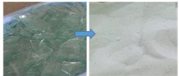
**Figure 1.** Waste glass sand after sieving in 0.08mm sieve
