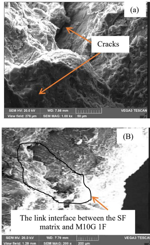
Figure 6. SEM of MC and M10G 1F mortars
