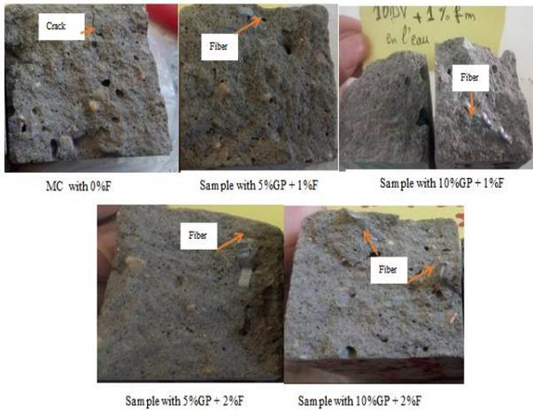
Figure 5. Surface of mortar after flexural strength test
