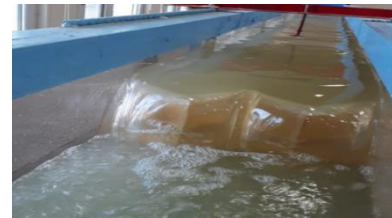
Figure 2. Triangular labyrinth weir with sharp crest after test
