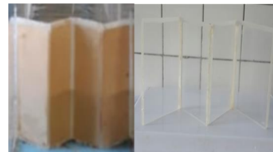
Figure 3. Triangular labyrinth weir with sharp crest before test
