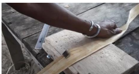
Figure 3. Palmyra leaves cutting tool developed by CSE R&D Team
