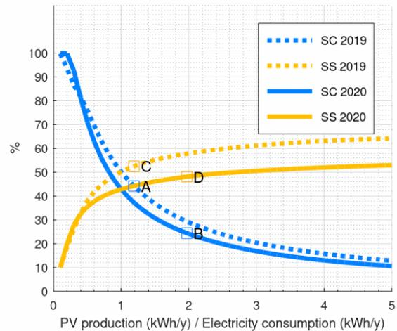
**Figure 13.** PV SC and SS rates in offices without BESS
