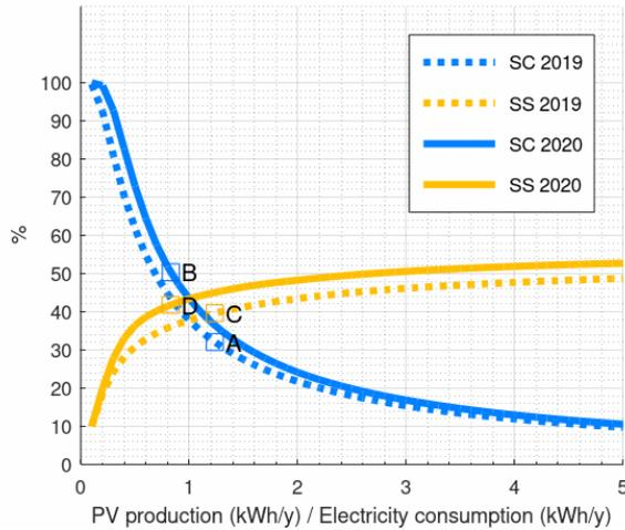
Figure 15. PV SC and SS rates in household without BESS
