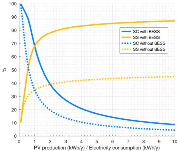
**Figure 8.** SC and SS in household without and with BESS of capacity/consumption = 1.5 kWh/MWh/y
