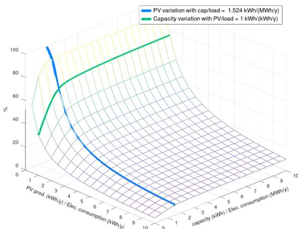
**Figure 9.** SC variation in household for different PV rated power and BESS capacity
