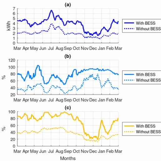
**Figure 12.** (a) Absolute self-consumption, (b) SC and (c) SS in household with and without BESS
