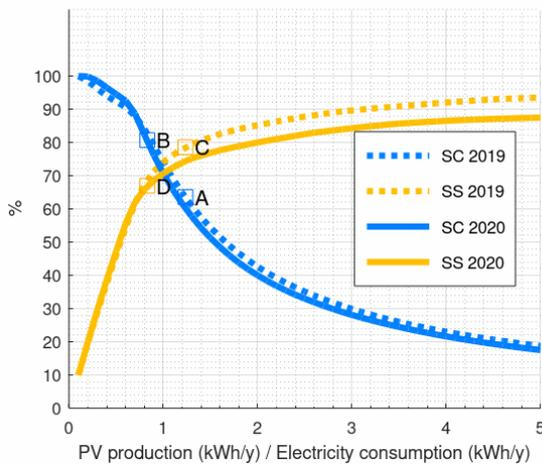
Figure 16. PV SC and SS rates in household with BESS
