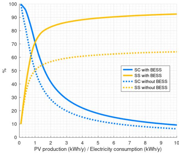
**Figure 3.** SC and SS in offices without and with BESS of ratio capacity/consumption = 1.0 kWh/MWh/y
