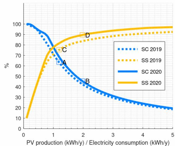
**Figure 14.** PV SC and SS rates in offices with BESS
