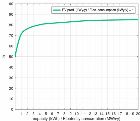
**Figure 5.** SC variation in office for different BESS capacities
