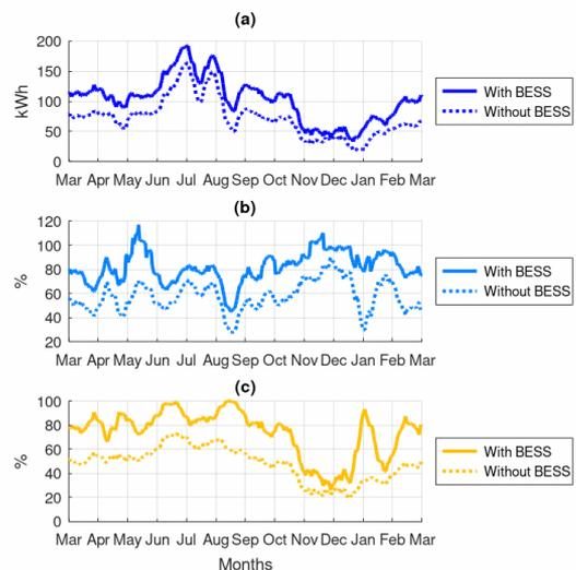
**Figure 11.** (a) Absolute self-consumption, (b) SC and (c) SS in office with and without BESS
