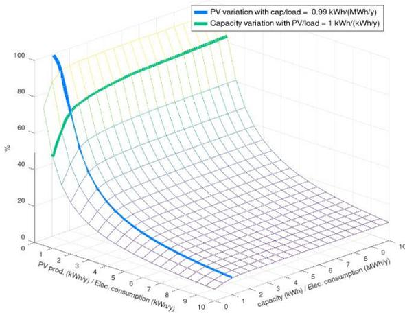
**Figure 4.** SC variation in office for different PV rated power and BESS capacity
