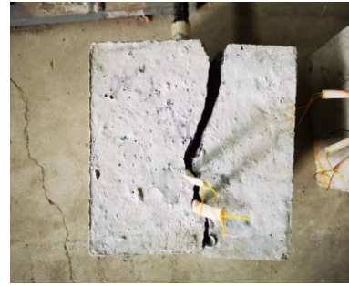
(2) Splitting damage of concrete
