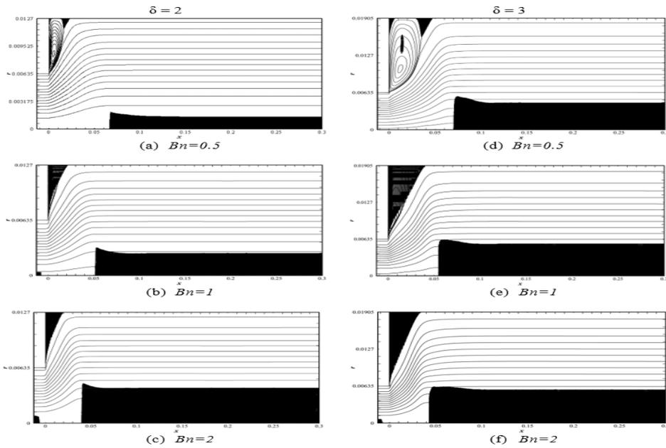
**Figure 11.** Stream function, yielded and un-yielded contours of non-Newtonian viscoplastic fluid at  $Re=50$
