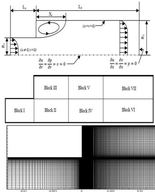
**Figure 1.** Sudden expansion geometry and mesh distribution near the 1:2 expansion (Mesh III,  $-d_1 < x < +d_1$  and  $0 < r < d_2$ )
