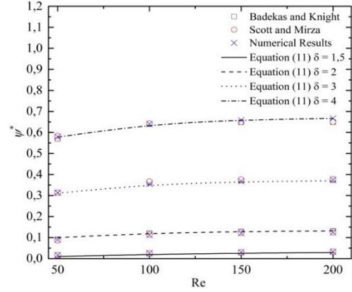
Figure 7. Eddy intensity  $\psi^*$  versus  $Re$  for  $Bn = 0$
