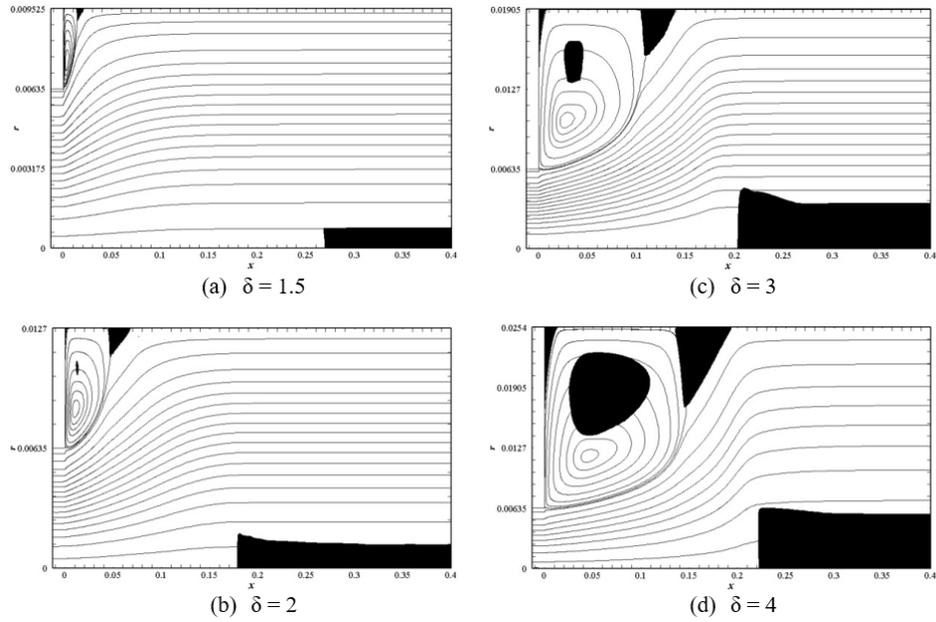
**Figure 10.** Stream function, yielded and un-yielded contours of non-Newtonian viscoplastic fluid at  $Re=150$  and  $Bn=0.5$
