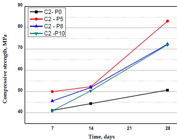
**Figure 6.** Compressive strength of C2 combination with and without pozzolan addition
