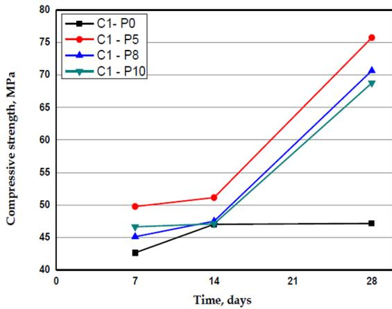
**Figure 5.** Compressive strength of C1 combination with and without pozzolan addition
