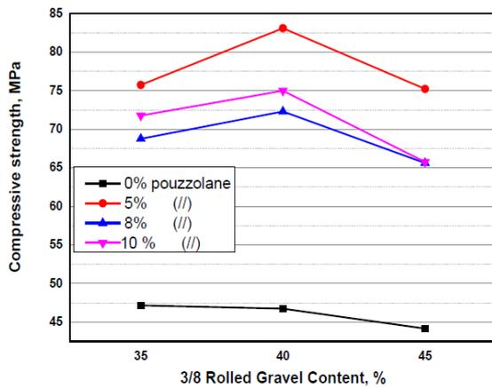
Figure 9. Effect of rolled gravel content on the compressive strength of concrete at 28 days
