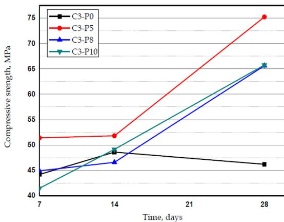
**Figure 7.** Compressive strength of C3 combination with and without pozzolan addition
