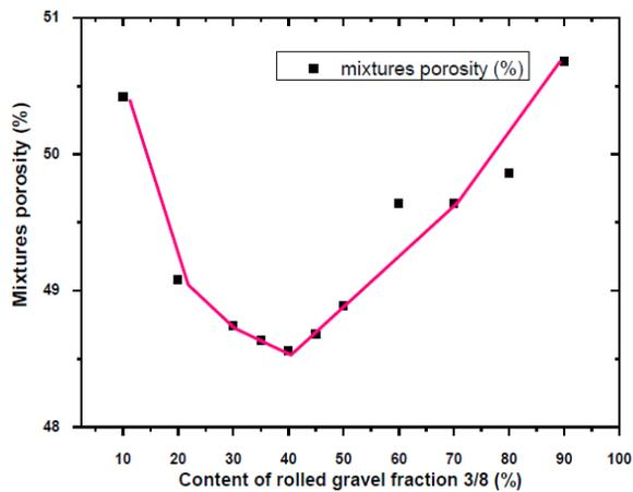
Figure 3. Porosity of mixtures gravel fractions
