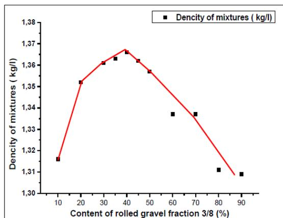
Figure 4. Density of mixtures of gravel fractions
