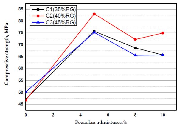
**Figure 8.** Compressive strength development depending on the percentage of pozzolan addition
