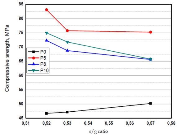
Figure 10. The relation between S/G ratio and the compressive strength
