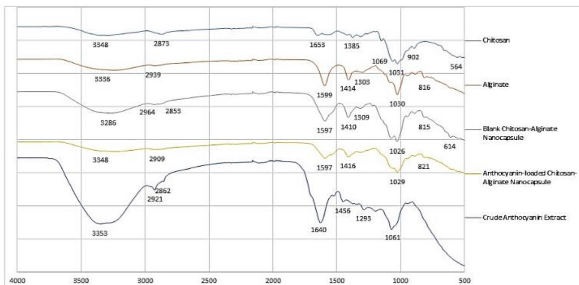
**Figure 4.** FTIR spectra of chitosan, alginate, blank chitosan-alginate nanocapsules (Blank CAN), anthocyanin-loaded chitosan-alginate nanocapsules (ALCAN), and crude anthocyanin extract (CAE) from fermented black garlic
