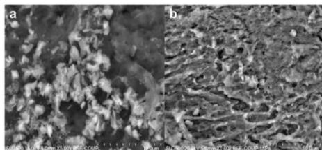
**Figure 3.** SEM images of a) blank chitosan-alginate nanocapsules (T0) and b) anthocyanin-loaded nanocapsules (T3)
