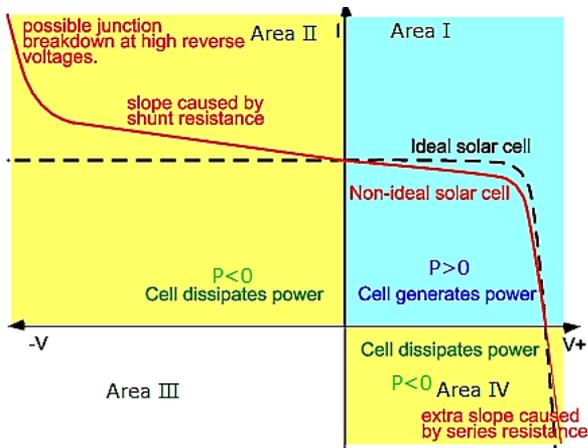
Figure 1. I-V characteristics with the operation mode in each
