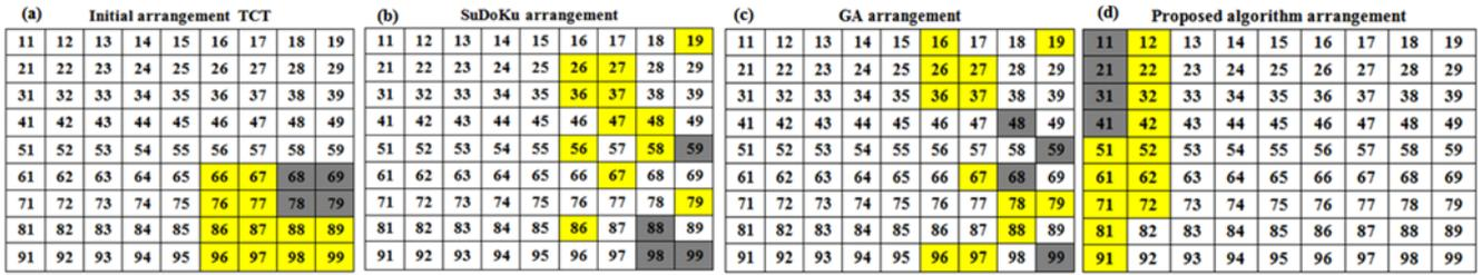
**Figure 21.** Shading pattern for case 7 (a) TCT interconnection scheme, (b)shade dispersion with Su Do Ku arrangement, (c)shade dispersion with GA arrangement, and (d) shade dispersion with Proposed arrangement
