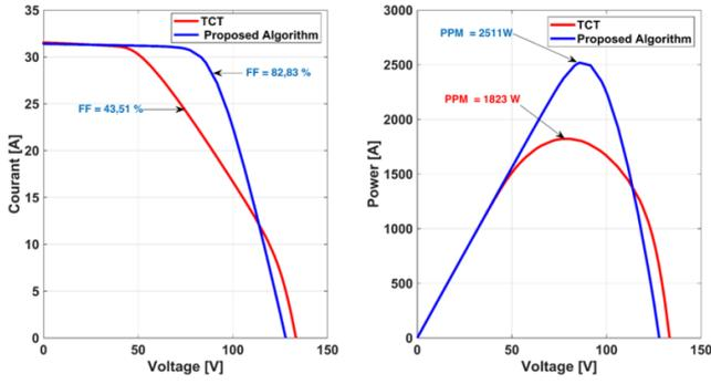
Figure 10. I-V and P-V characteristic curve for case 1
