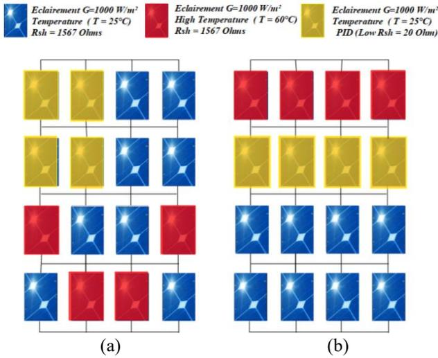
Figure 11. PV array under 50% of infected modules, (a) TCT configuration, (b) proposed algorithm arrangement
