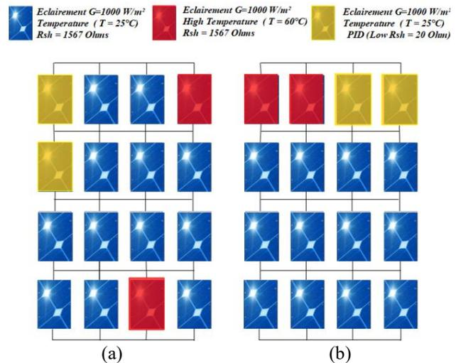
**Figure 9.** PV array under 25% of infected modules, (a) TCT configuration, (b) proposed algorithm arrangement
