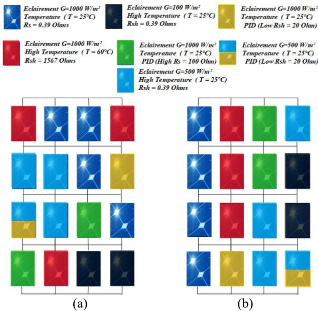
Figure 17. PV array under 75% PV modules infected, (a) TCT configuration, (b) proposed algorithm arrangement
