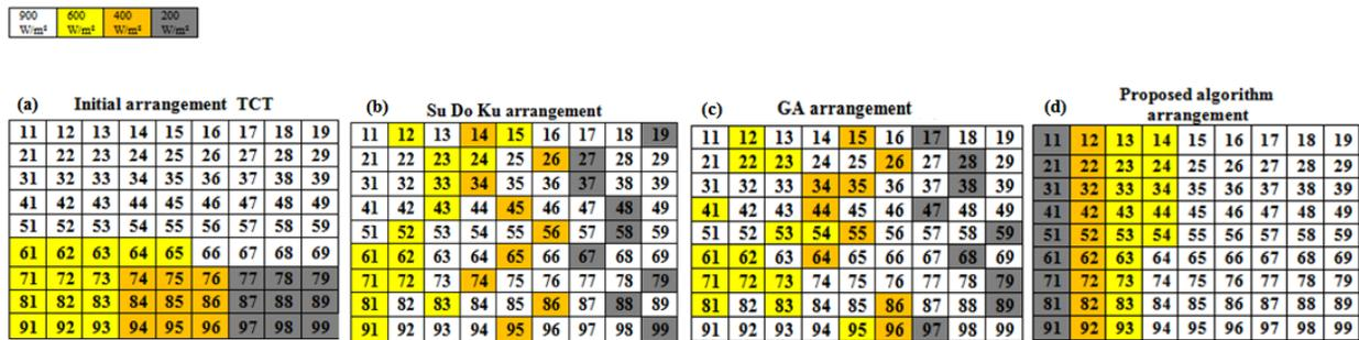
**Figure 19.** Shading pattern for case 6 (a) TCT interconnection scheme (b) shade dispersion with Su Do Ku arrangement, (c) shade dispersion with GA arrangement, and (d) shade dispersion with proposed arrangement
