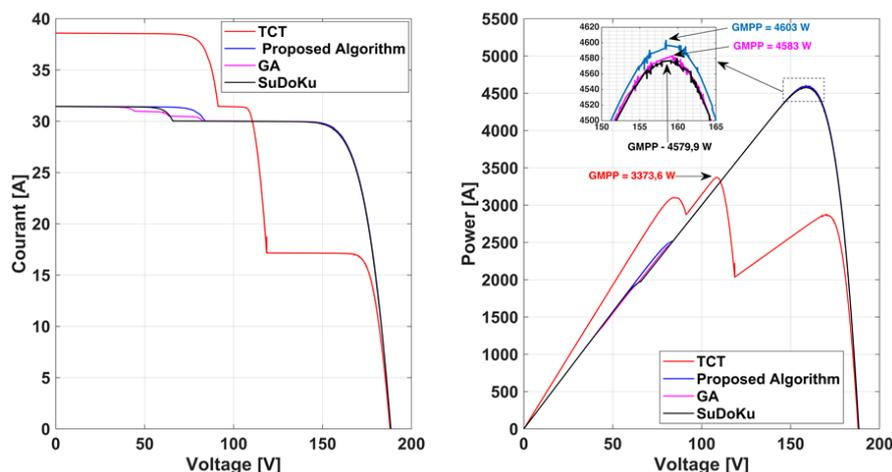
**Figure 20.** I-V and P-V characteristic curve for case 6
