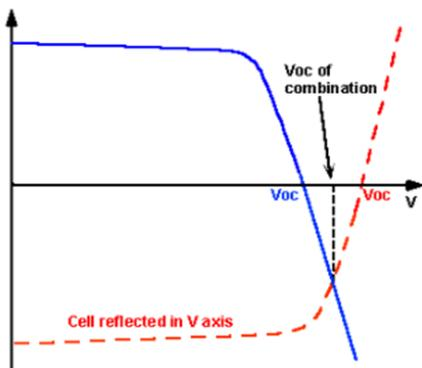
**Figure 5.** A graphical way to calculate the combined voltage
