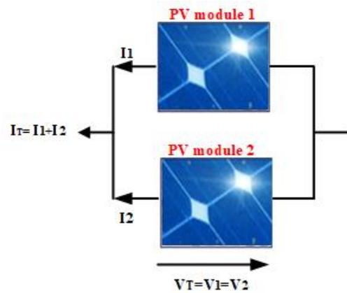
Figure 2. PV cells in parallel connection without a mismatch issue
