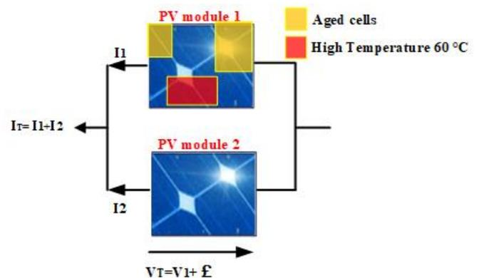
Figure 3. PV cells in parallel connection with a voltage mismatch
