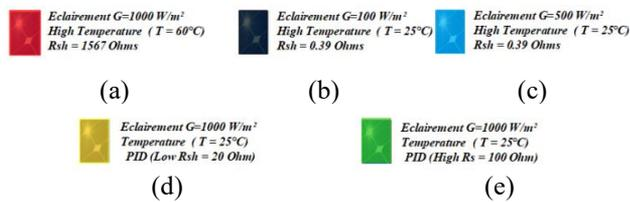
**Figure 8.** Different phenomena can be found, (a) high temperature, (b) partial shading (100w/m<sup>2</sup>), (c) partial shading (500w/m<sup>2</sup>), (d) a decrease in the parallel resistance and (e) an increase in the series resistance
