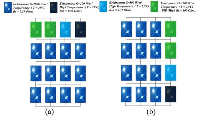
Figure 13. PV array under 25% of infected modules, (a) TCT configuration, (b) proposed algorithm arrangement
