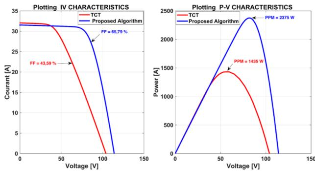
Figure 12. I-V and P-V characteristic curve of case 2
