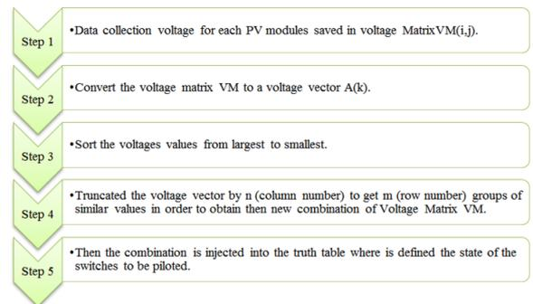
**Figure 7.** Main steps of the voltage balancing algorithm
