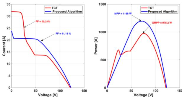
Figure 18. I-V and P-V characteristic curve for case 5
