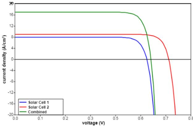
**Figure 4.** I-V curve example of two PV cells connected in parallel with a voltage mismatch
