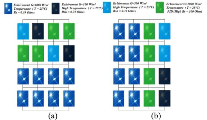
Figure 15. PV array under 50% of infected modules, (a) TCT configuration, (b) proposed algorithm arrangement
