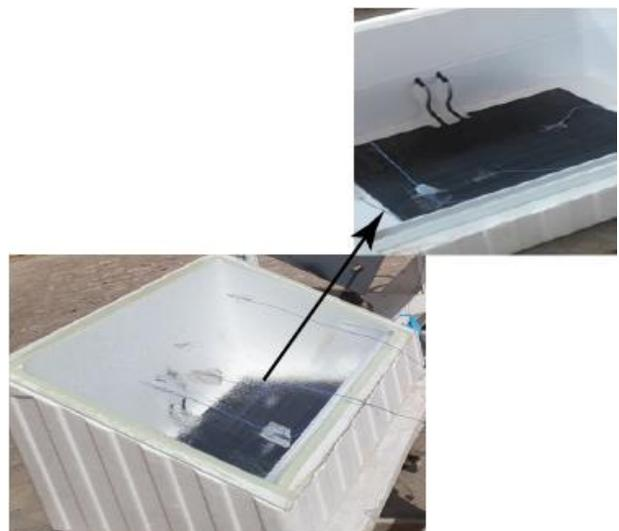
**Figure 2.** Single solar still with heat exchanger
