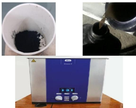
**Figure 4.** Preparation of nanofluid; Elma ultrasonic device and Copper Oxide (CuO)
