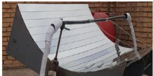
**Figure 1.** Photograph for the parabolic trough solar collector with the receiver tube
