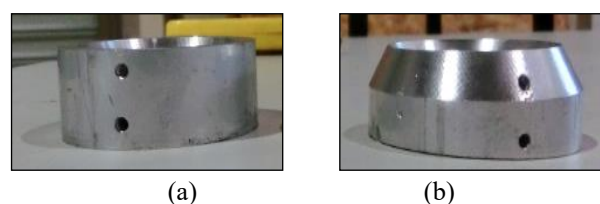
Figure 2. Fuel pan (a) 0° and (b) 60° pan wall angle
