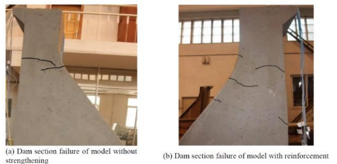
Figure 2. Dam section failure patterns under the earthquake [19]
