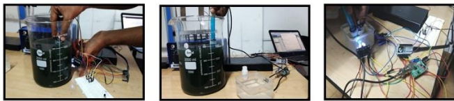
Figure 4. Measurement of Colour, Turbidity and pH during Electrocoagulation Process in Batch Mode using IoT
