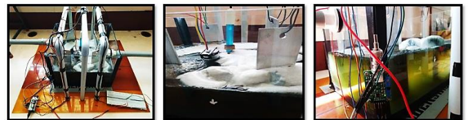
Figure 7. Measurement of Colour, Turbidity and pH during Electrocoagulation Process in Modified Batch Mode using IoT
