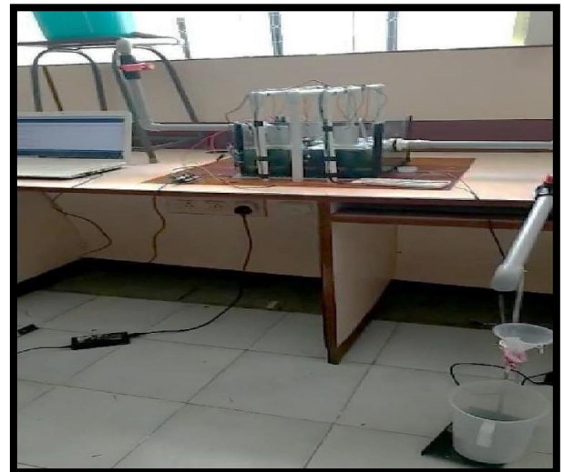
Figure 6. Experimental Setup for Electrocoagulation Process in Modified Batch Mode using IoT
