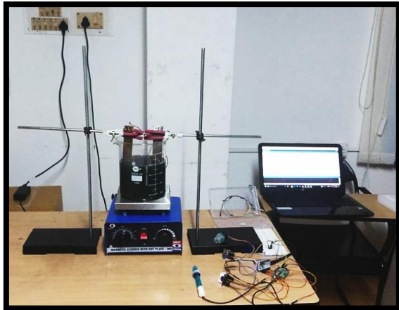
Figure 3. Experimental Setup for Electrocoagulation Process in Batch Mode using IoT
