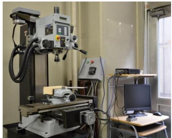
**Figure 5.** An appearance of CNC milling machine (PSF550-CNC)
