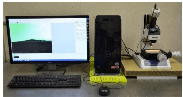
**Figure 9.** A system configuration of optical microscope with a specimen
