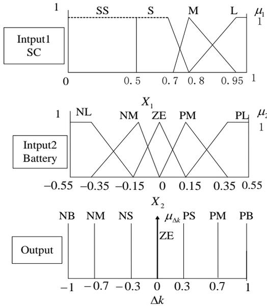
**Figure 1.** Membership functions of  $X_1(t)$ ,  $X_2(t)$  and output ( $\Delta p(t) \geq 0$ )
