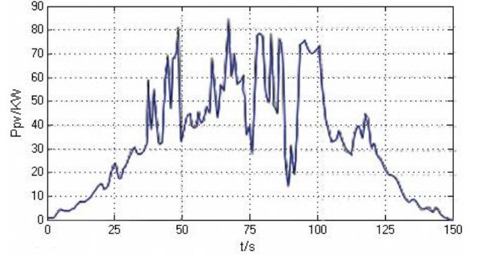
**Figure 4.** Output power waveform of PV power generation system
