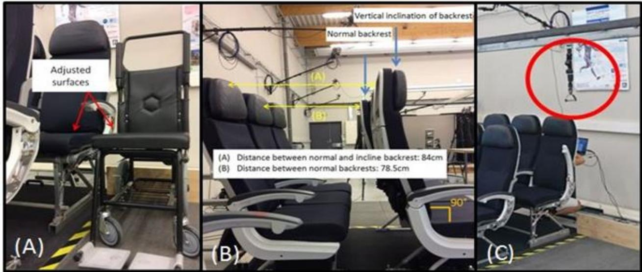
**Figure 1.** Adaptations on the aircraft seat and on the boarding chair
