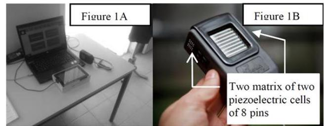
**Figure 1.** A: The Tactos system. Here, for a left-handed person, the tactile interaction module is to the right of the touch pad. B: The Tactile Interaction Module with matrix of two Braille cells
