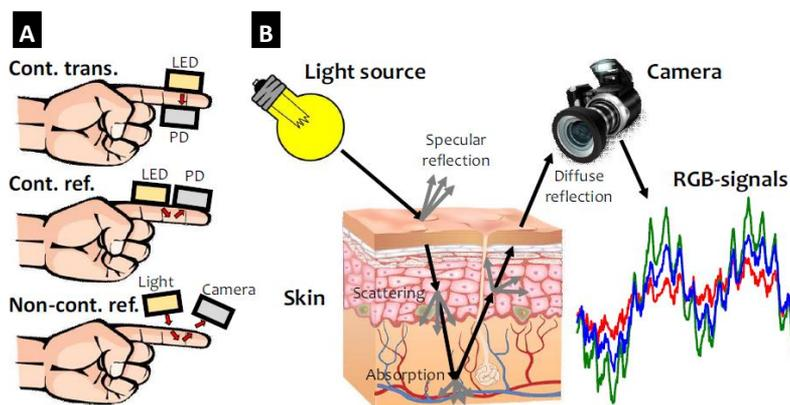
**Figure 4.** (A) Photoplethysmography consists in measuring variations in light absorption on skin tissues. (B) The RGB signals (one per chromatic component of the camera sensor) contain typical pulse waves whose shape depends on diastolic and systolic phases. From [17]
