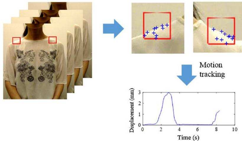
**Figure 5.** Breathing process produces a slight movement of the shoulders that can be tracked from video streams recorded by a camera. Computer vision techniques can be deployed to detect and track relevant features on the shoulders. A time signal that reflects the displacements, and thus inspiration and expiration phases, is computed from the tracked points. Modified from [35]
