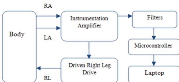
**Figure 2.** Block diagram of ECG acquisition system
