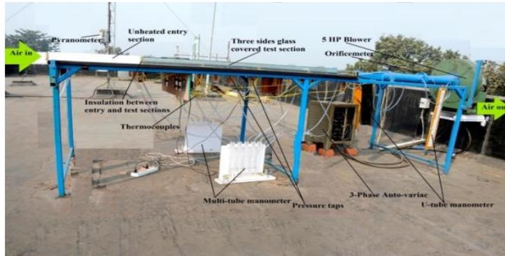
Figure 2. Photograph of test setup
