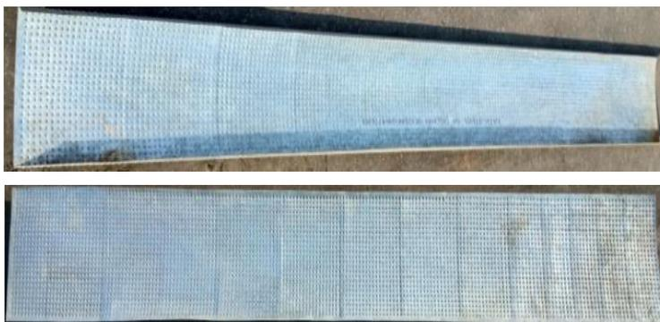
Figure 4. Photograph of one and three sides roughened absorber plates
