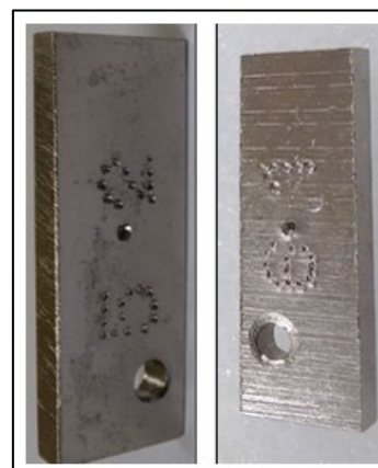
Figure 4. The NiP coupons with 67.40 µm do not show partial destruction because of the attack of HCl at 60 °C and 4 h of immersion
