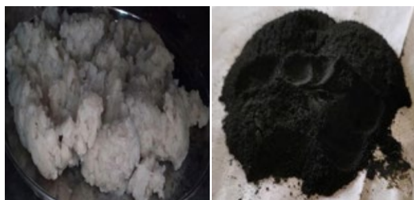
Figure 1. Dried orange peels, banana peels, potato starch and derived activated carbon
