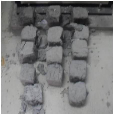
Figure 3. The state of the test specimen when it reaches the ultimate strength
