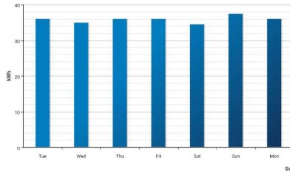
Figure 24. Real SOFC week production on the site of installation
