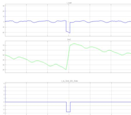
Figure 21. Behavior of the system (*I<sub>batt</sub>, SoC, I<sub>to Grid\_DC\_side</sub>*) July, current control mode, maximum SOFC set point
