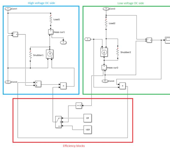
Figure 10. Bidirectional DC/DC model (current control)
