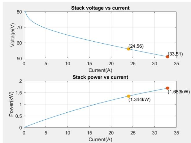
Figure 4. SOFC simulated curves
