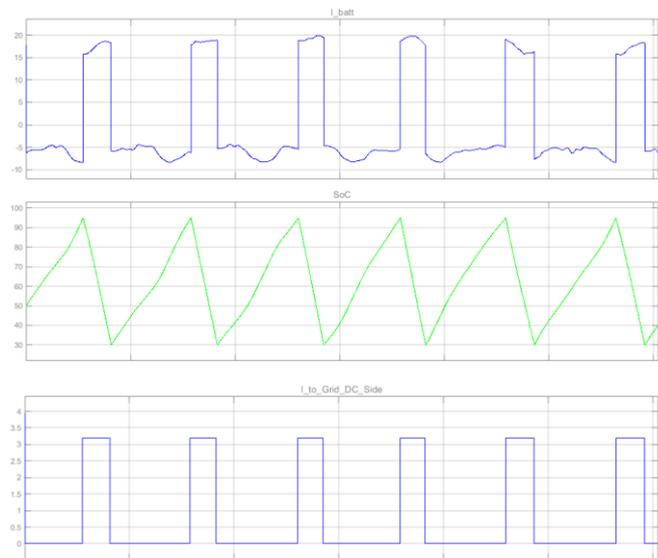
Figure 18. Behavior of the system ( $I_{batt}$ , SoC,  $I_{to\_Grid\_DC\_side}$ ) March, current control mode
