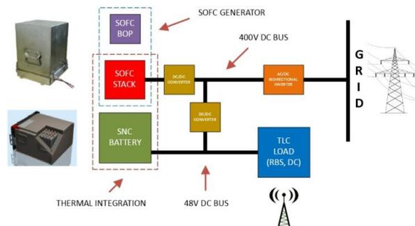
Figure 2. Hybrid system configuration
