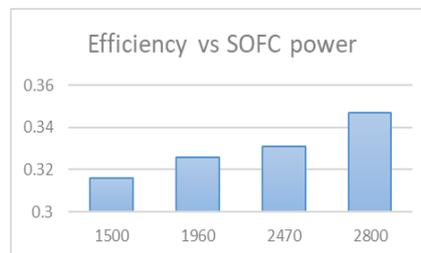
*Figure 23. System efficiency variation with different SOFC set points*
