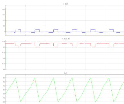
Figure 20. Behavior of the system ( $I_{batt}$ ,  $V_{bus\_48}$ , Soc), March, voltage control mode
