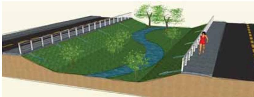
Figure 7: Sinuous channel in a green alley as an alternative to the traditional pipes.
