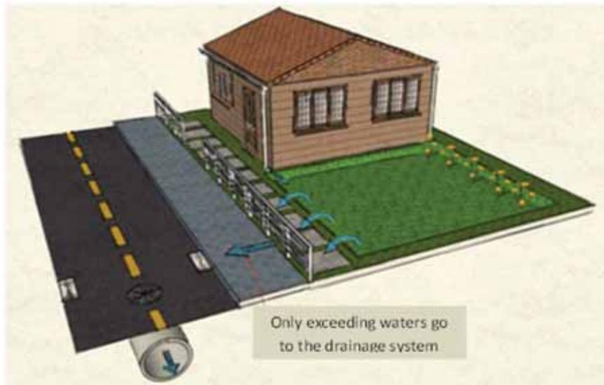
Figure 5: Lots occupation considering a storage and infiltration capacity in the garden area — disconnection from the formal drainage system.
