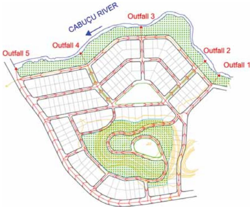
Figure 4: Traditional drainage system designed for the new housing subdivision area.
