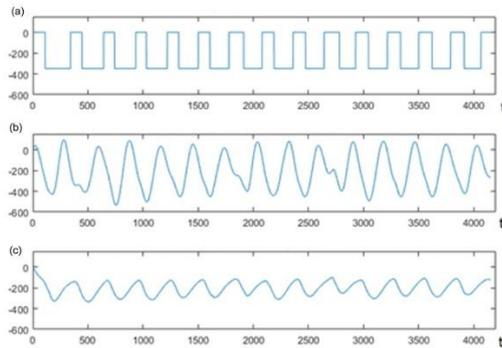
Figure 8. Electrical consumptions with three different controller types: (a) ON/OFF; (b) PID; (c) MPC
