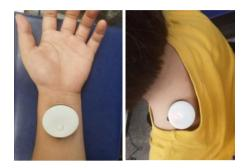
Figure 15. The photos of the proposed wearable ESR device
