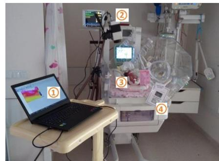
Figure 2. Measurement setup: (1) portable computer, (2) infrared camera, (3) neonate, and (4) incubator
