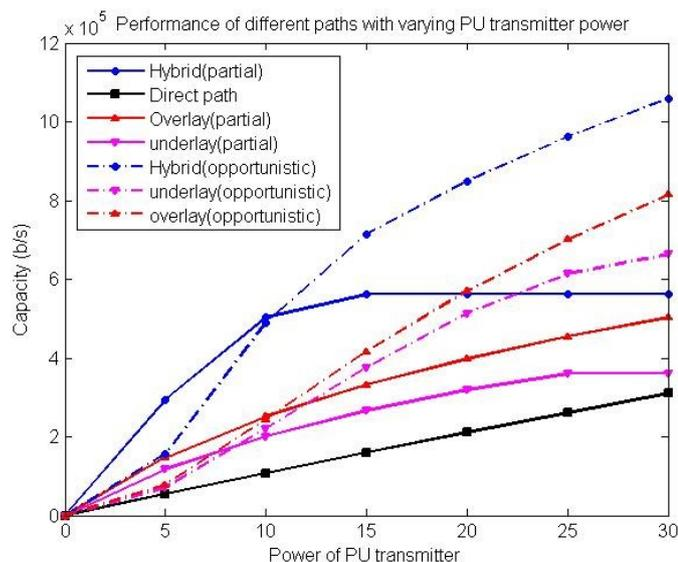
**Fig.5.** Capacity over different paths with partial and opportunistic relay selection and fixed Interference threshold.
