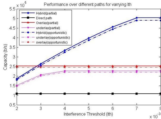
**Fig.4.** Capacity over different paths with partial and opportunistic relay selection and fixed PU transmitting power.
