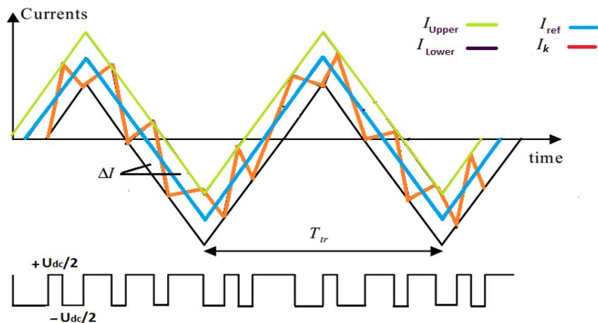
Fig.6. Simplified diagram of hysteresis band current controller
