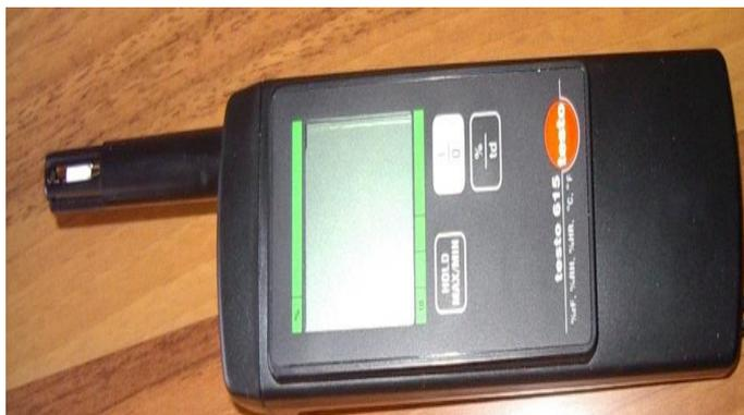
Figure 2. Thermo-hygrometer and thermo-anemometer
