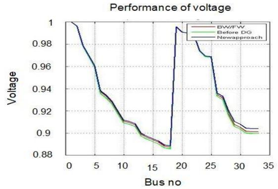
Figure 7. Performance of voltage by new approach after DG connected
