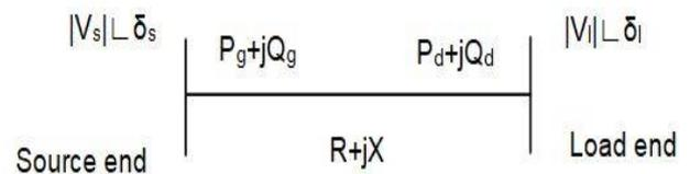
**Figure 1.** Single line diagram of a simple radial distribution system
