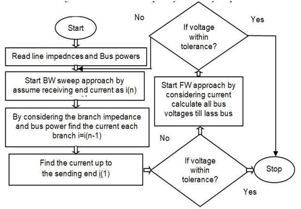
Figure 2. Flowchart for BW/FW sweep approach
