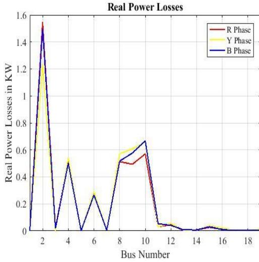
Figure 6. Real power losses at each bus
