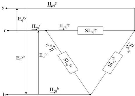
Figure 2.  $\Delta$ -Connected load model
