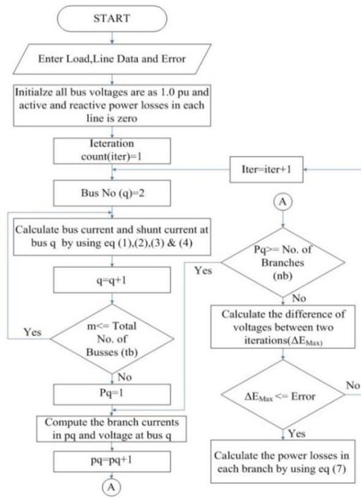
Figure 4. Flow Chart for Unbalanced Load flow of URDNs
