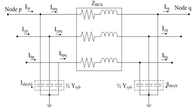
Figure 3. Distribution system line model
