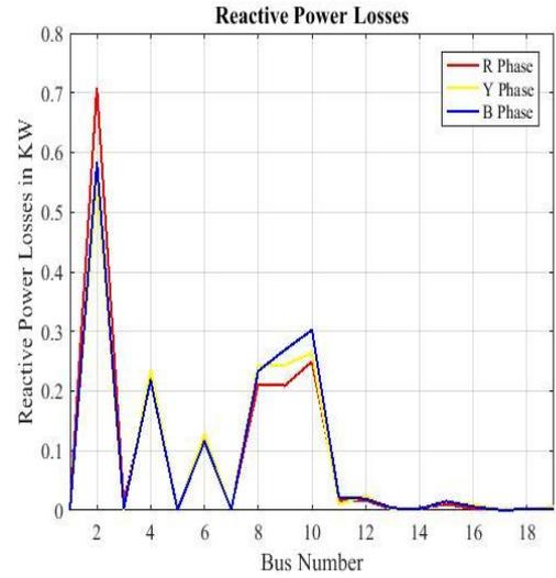
Figure 7. Reactive power losses at each bus
