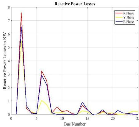
Figure 10. Reactive power losses at each bus
