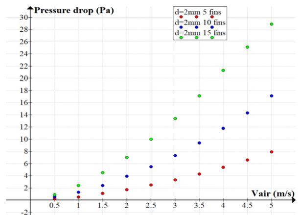
Figure 13. Pressure drop of air through the pin heat sink in different square configurations
