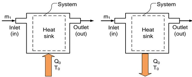
Figure 1. Schema of the heat exchange in the heat sink
