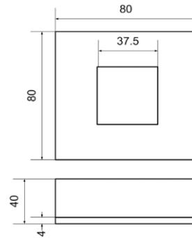
Figure 7. Dimensions of heat sink and heat source
