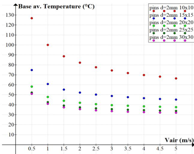
Figure 9. Average base temperature of the pin heat sink in different square configurations
