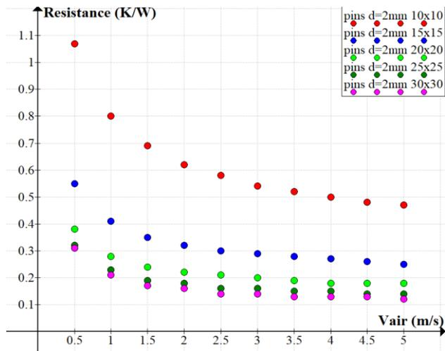
Figure 8. Thermal resistance of the pin heat sink in different square configurations
