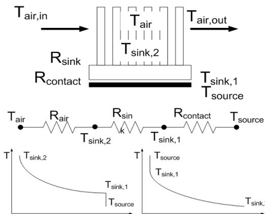
**Figure 5.** System schema and electric analogy with representation of cooling and heating case
