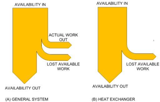
Figure 2. Energy transformation in a general mechanic system and in a heat exchanger
