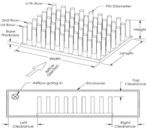
**Figure 4.** Round pin heat sink schematic drawing
