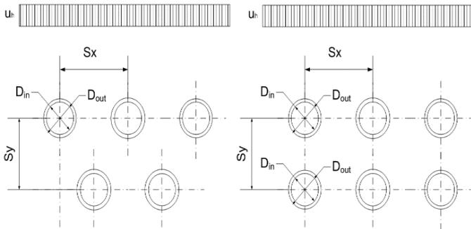
Figure 6. Staggered and inline configurations
