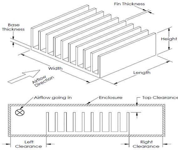
**Figure 3.** Fin heat sink drawing
