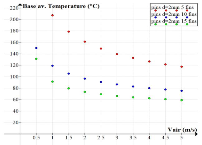
Figure 12. Average base temperature of the fin heat sink in different configurations
