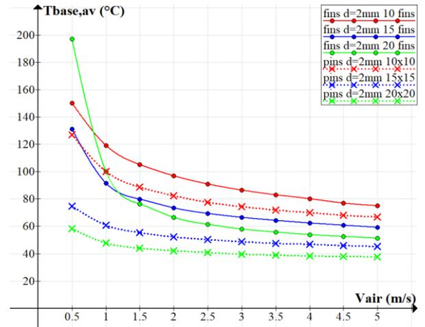
**Figure 16.** Comparison between finned and pin heat sinks in terms of heat dissipation capability
