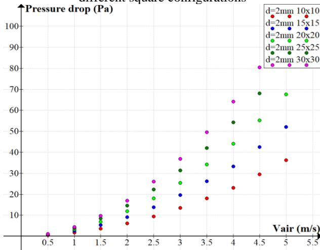
Figure 10. Pressure drop of air through the pin heat sink in different square configurations
