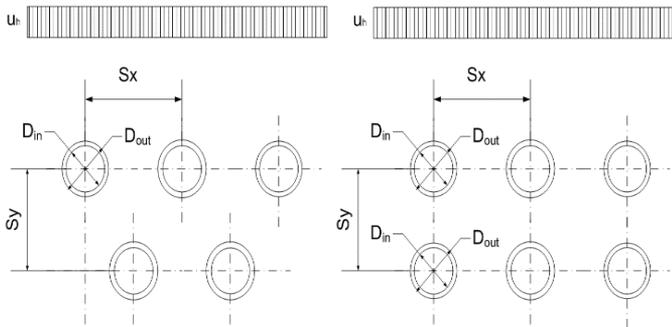
Figure 6. Staggered and inline configurations
