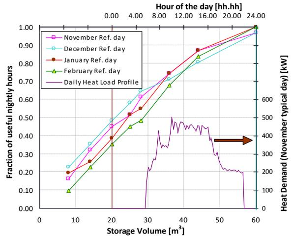
**Figure 5.** Fraction of nightly hours in cogeneration mode by the CGTs as a function of the storage volume. Typical days per month are considered in terms of temporal heat demand profile. Second axes: typical November day heat profile
