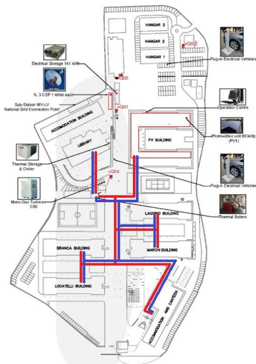
**Figure 1.** The layout of the SPM at the Savona Campus of the University of Genova, Italy. Photovoltaic strings (PV), Cogenerative Gas Turbines (CGT), back up Gas Heater (GH), Electric Storage (ES). The red and blue lines represent the thermal network that fed the Campus
