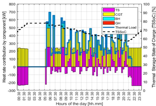
**Figure 4.** Heat transfer rate contributions by component as a function of time for the 26<sup>th</sup> of February, 2017. Negative values represent the charging periods of the TS. On the secondary axis the TS state of charge is represented. Storage volume 60m<sup>3</sup>
