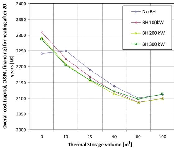
**Figure 6.** Overall cost for heating system (TS and BH) after 20 years of operations
