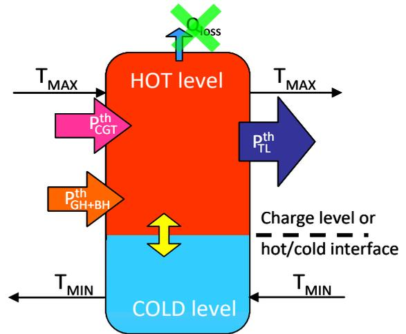
**Figure 2.** Thermal storage model. The open system is described as an energy storage of battery type where only two temperature levels are present
