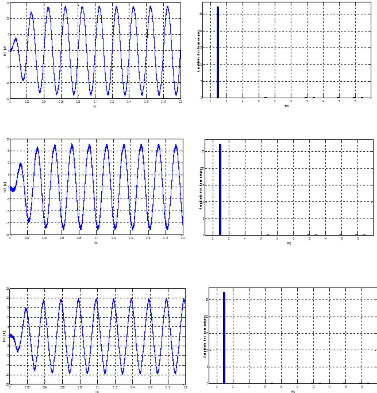
**Figure 12.** Source currents after filtering and their frequency spectra using Fuzzy Logic controller
