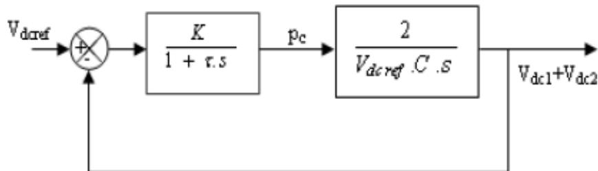
Figure 6. Dc voltage control block
