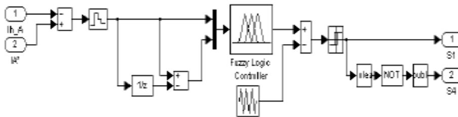
Figure 5. Generation process of switching signals
