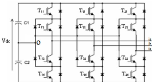
**Figure 2.** Structure of three-level voltage inverter
