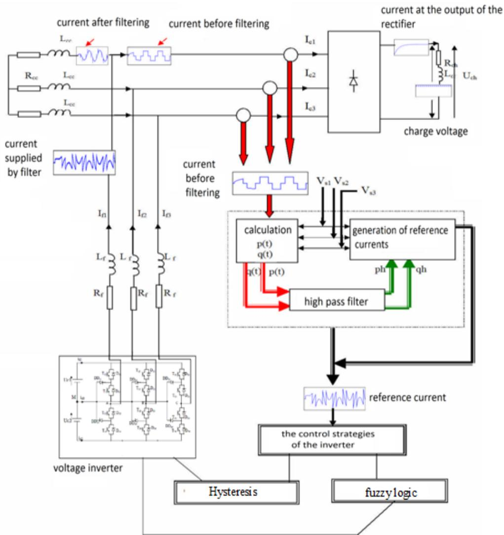
**Figure 1.** Active power filter operation
