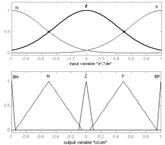
Figure 4. Membership function for the inputs and output variables
