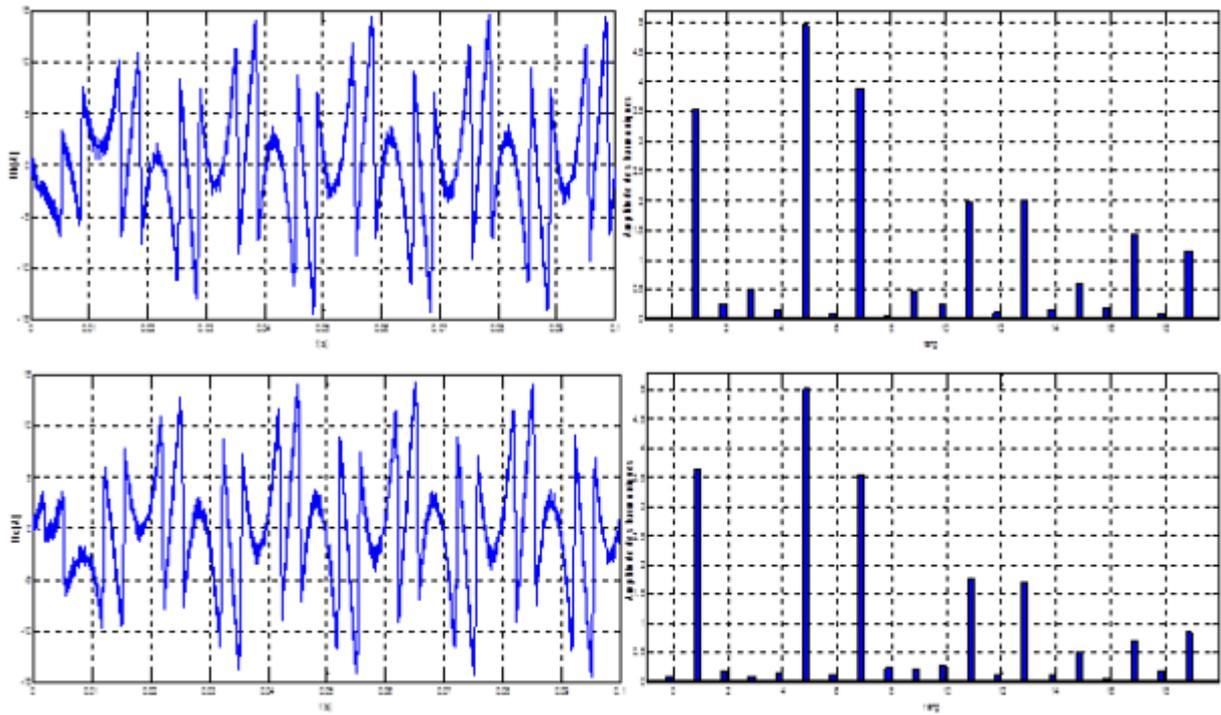
**Figure 7.** Currents injected by the inverter and their frequency spectra for the hysteresis control ( $\Delta h = 0.1$  A)
