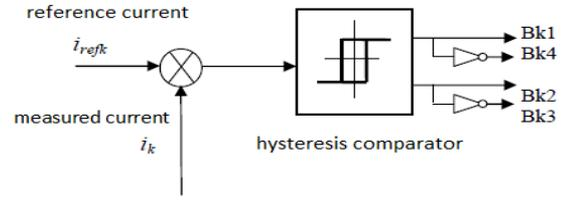
Figure 3. Principle of current control by hysteresis
