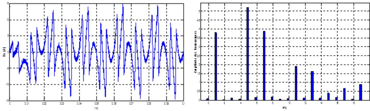
**Figure 10.** Currents injected by the inverter and their frequency spectra using Fuzzy Logic controller
