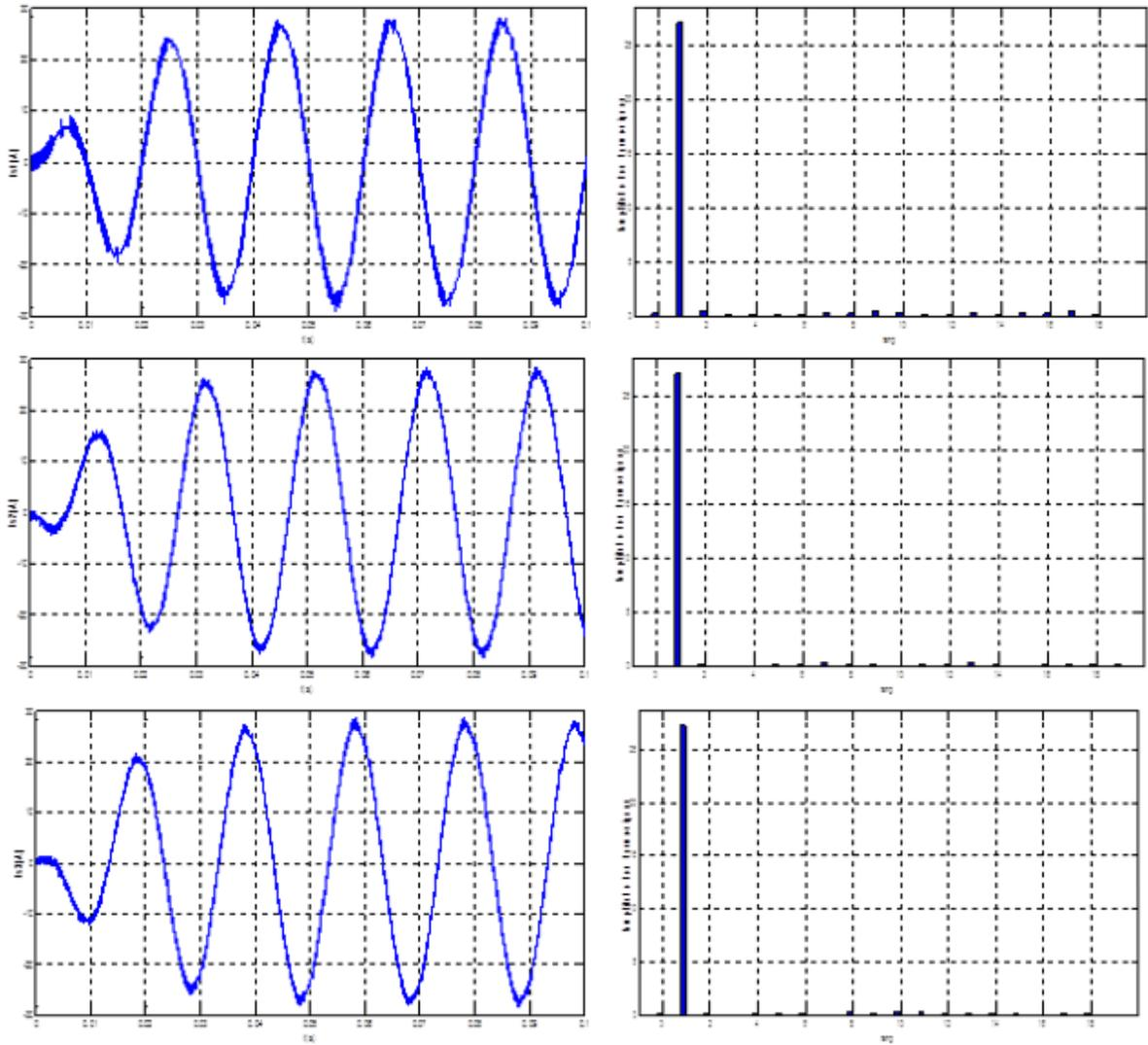
**Figure 9.** Source currents after filtering and their frequency spectra for the hysteresis control ( $\Delta h = 0.1$  A)
