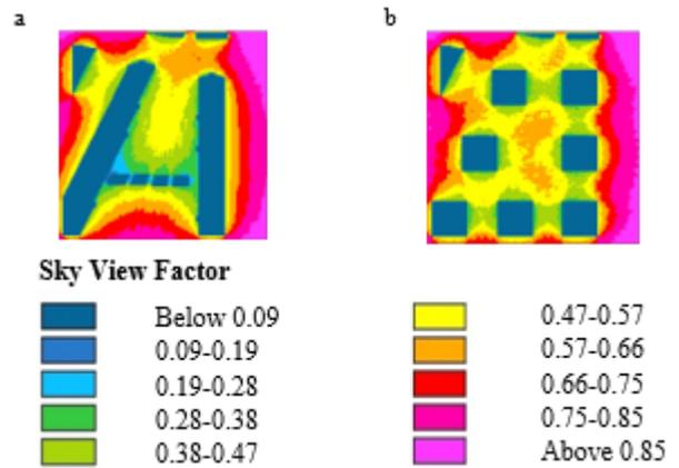
**Figure 8.** SVF - Scenarios Comparison at 13:00, h=1.5 m: a) BaseS, b) TowerS
