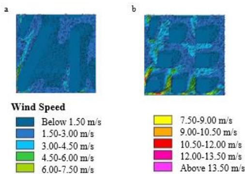
**Figure 6.** Wind Speed [m/s] - Scenarios Comparison at 13:00, h=1.5 m: a) BaseS, b) TowerS
