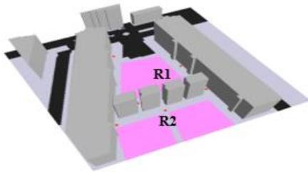
Figure 1. Base Scenario 3D model in ENVI-met with the receptors positions
