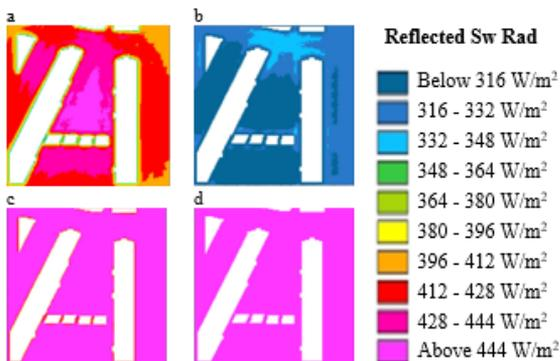
**Figure 7.** Reflected Sw Radiation [W/m<sup>2</sup>] - Scenarios Comparison at 13:00, h=1.5m: a) BaseS, b) Green S, c) BlueWS, d) WhiteBS
