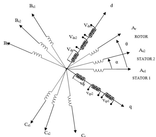
Figure 1. Doubly stator winding representation
