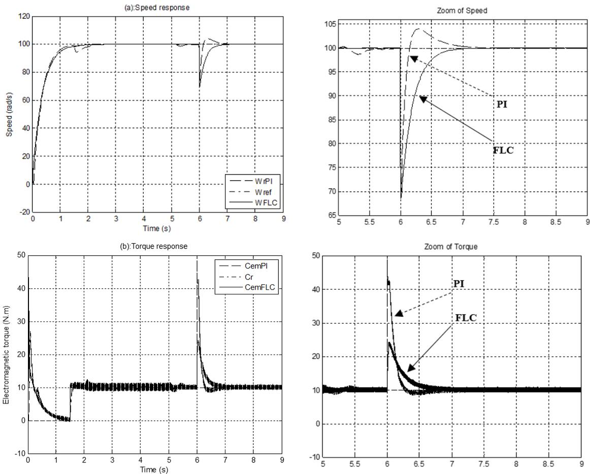
**Figure 8.** Speed and torque characteristic of an (DFOC) with PI and FLC controllers, at parametric variations (rotor resistance ( $R_{r1}=1.5*R_r$ ), moment of inertia ( $J_1=1.5*J$ )).
