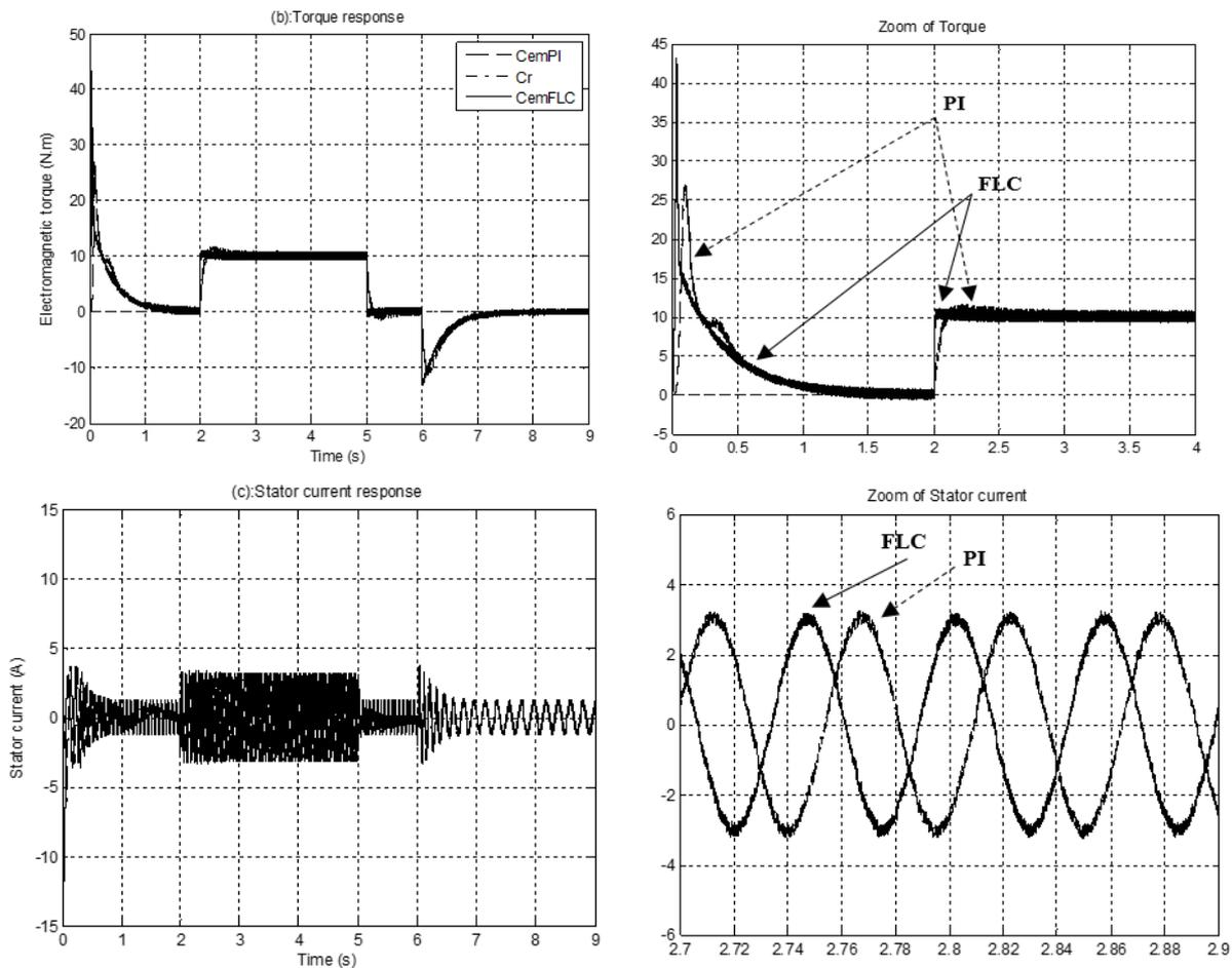
**Figure 6.** Speed, torque and current stator characteristic of an (DFOC) with PI and FLC
