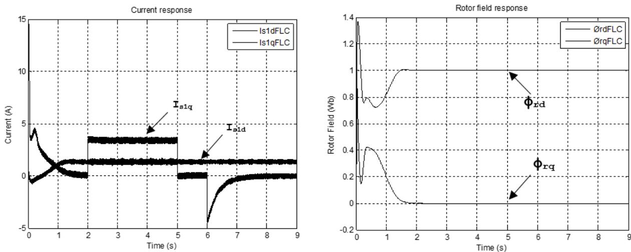
**Figure 7.** Decoupling and rotor field orientation
