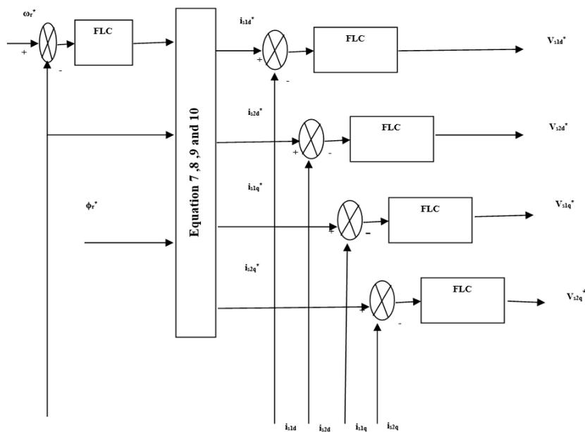
Figure 4. Block diagram of the fuzzy logic PI controller for DFOC approach of the DSIM
