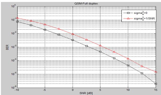
Figure 3. BER of QSM based FD
