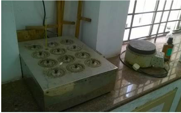
Figure 3. Electroless Plating Setup
