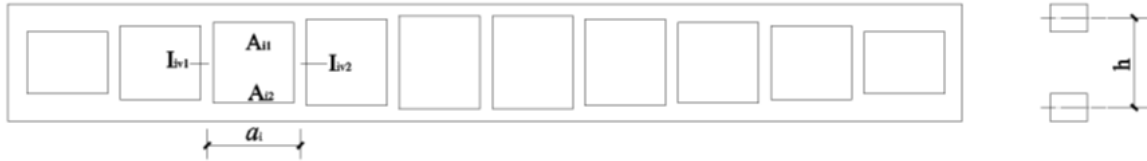
Figure 1. The Vierendeel truss and its typical internode
