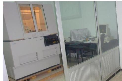
**Figure 3.** Philips X-ray diffractometer photo
