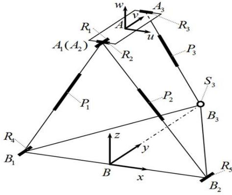
Figure 1. The type of 2-RPU&SPR PM
