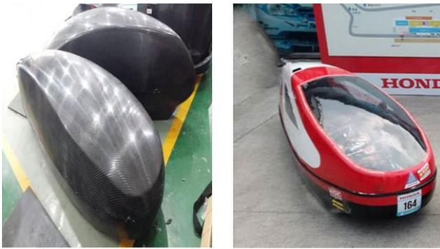
Figure 15. The production of finished carbon fiber body
