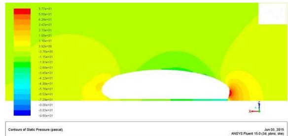
**Figure 12.** The distribution of pressure in the body of the vehicle body
