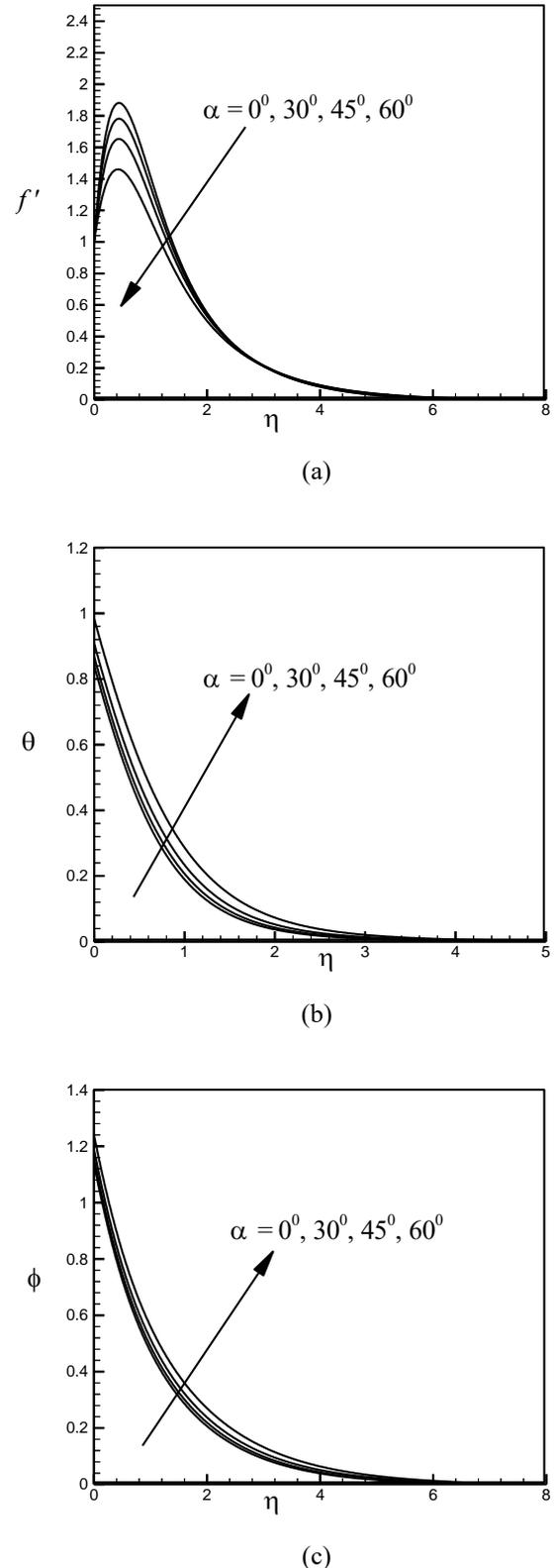
**Figure 2.** Dimensionless (a) velocity, (b) temperature and (c) concentration profiles for different values of  $\alpha$
