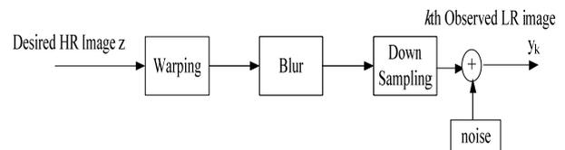
**Figure 1.** Observation model of super-resolution reconstruction
