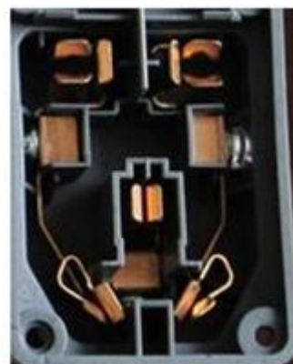
Figure 1. Internal structure diagram of socket
