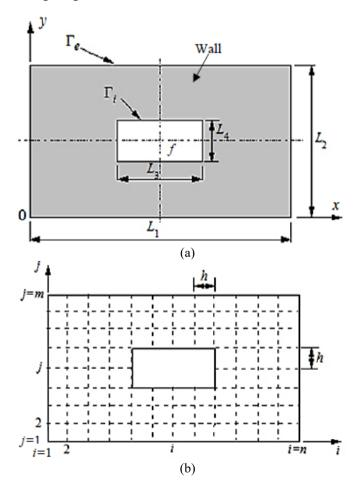
Figure 1. (a): Geometry and (b): grid of the walls of the Oven
