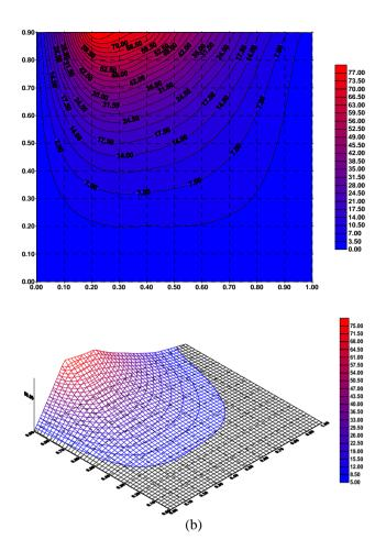
**Figure 2.** Winding of isothermals (a) and (b) for  $T_{L'} = T_{0'} = 0$ , without source
